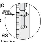
ring on the Titrator meets the Titrator barrel. Record as ppm Sodium Nitrite ( $\text{NaNO}_2$ ).
